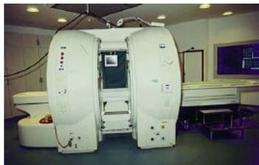
Figure 2. Open, whole body MRI magnet (Signa SP/i 0.5 T, General Electric Medical Systems, Milwaukee, WI, USA)
