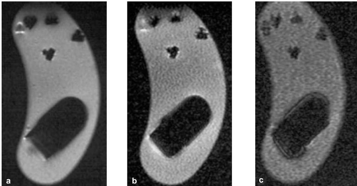
**Figure 4.** Artifact diagnostic in an vertical open, whole body MRI-system (Signa SP/i, 0.5 T, GE Medical Systems, WI, USA) - in glycerol gelatine embedded material of aluminum and brass. Examinations with varying sequences: a) fast spin-echo pulse sequence, b) spin-echo pulse sequence, c) gradient echo pulse sequence.
